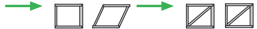
A rectangular structure (such as a wall frame) can deform without bracing
